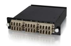
Small form factor: 1.125in x 5.125in x 4.5in. This breakout module provides the mechanical distribution of two 12-strand MTP/MPO connectors. Housed in a rugged steel enclosure guaranteed for life, this durable module arrives fully loaded with the preterminated and tested MTP/MPO breakout harness. It is shipped with a test report that can assist in calculating the optical budget.
