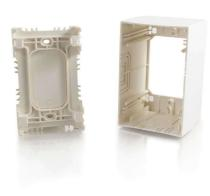
Extra deep design accommodates the demands for cabling with full size connectors and eliminates congestion. Convenient break-away ports on all four sides accommodate flexible installation of up to four different raceway sizes! Two inches of depth offers less congestion from bend radii during wall plate installation.
