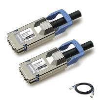
This is a MSA Compliant 10GBase-CU CX4 to CX4 direct attach cable that operates over passive copper with a maximum reach of 3.0m (9.84ft). It has been programmed, uniquely serialized, and data-traffic and application tested to ensure it is 100% compliant and functional. Legrand direct attach cables are built to comply with MSA (Multi-Source Agreement) standards. All Legrand twinax and AOC cables are Trade Agreements Act (TAA) compliant.
