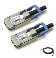
This is a MSA Compliant 10GBase-CU CX4 to CX4 direct attach cable that operates over passive copper with a maximum reach of 3.0m (9.84ft). It has been programmed, uniquely serialized, and data-traffic and application tested to ensure it is 100% compliant and functional. Legrand direct attach cables are built to comply with MSA (Multi-Source Agreement) standards. All Legrand twinax and AOC cables are Trade Agreements Act (TAA) compliant.
