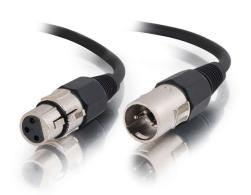
Use this XLR to XLR cable to connect unbalanced sources to balanced XLR inputs. This pro-audio cable is made from 22 AWG twisted pair audio cable under an aluminum foil shield and 60% copper braid for maximum shielding from noise. The highly flexible 7mm PVC jacket reduces the risk of the cable kinking and damaging the conductors.
