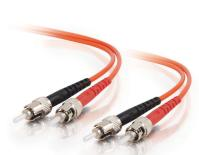
With ST to ST termination, this high quality fiber optic patch cable is specifically designed for ethernet, multimedia, or communication applications. The ST connector features a bayonet locking system. The plenum rating provides the fire protection required to run this cable within walls and air plenums without using conduit. The patented injection molding process provides each connection greater durability in resisting pulls, strains and impacts from cabling installs.
