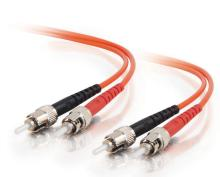
With ST to ST termination, this high quality fiber optic patch cable is specifically designed for ethernet, multimedia, or communication applications. The ST connector features a bayonet locking system. The plenum rating provides the fire protection required to run this cable within walls and air plenums without using conduit. The patented injection molding process provides each connection greater durability in resisting pulls, strains and impacts from cabling installs.
