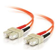
With SC to SC termination, this high quality fiber optic patch cable is specifically designed for ethernet, multimedia, or communication applications. The SC connector features a push-pull locking system. The plenum rating provides the fire protection required to run this cable within walls and air plenums without using conduit. The patented injection molding process provides each connection greater durability in resisting pulls, strains and impacts from cabling installs.
