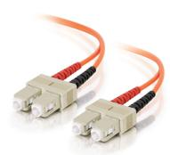
With SC to SC termination, this high quality fiber optic patch cable is specifically designed for fast ethernet, fiber channel, ATM and gigabit ethernet applications. The SC connector features a push-pull locking system. The LSZH jacket is composed from materials that lessen the smoke and halogen emissions when the cable is exposed to extreme temperatures.
