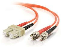
With SC to ST termination, this high quality fiber optic patch cable is specifically designed for fast ethernet, fiber channel, ATM and gigabit ethernet applications. The SC connector features a push-pull locking system while the ST connector features a bayonet locking system. The LSZH jacket is composed from materials that lessen the smoke and halogen emissions when the cable is exposed to extreme temperatures.
