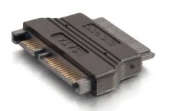
The Micro Sata to Sata adapter converts the connection commonly found on 1.8 inch solid state drives to Sata connections. This adapter will allow for both the power and data connecitons to convert to standard Sata connectors to allow the 1.8 inch SSD to connect in a PC. This adapter will also allow the 1.8 inch SSD to convert to a USB to SATA adapter to pull information off the drive.
