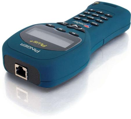
The Pinger Plus can PING using variable packet sizes and up to 99 times consecutively. In addition, PING can be performed for a single IP address, or a range of IP addresses. The Pinger Plus also identifies reversed polarity for improperly connected wire pairs, and provides a port ID feature with selectable blink rates to identify to which port on a hub or switch the wall outlet is connected.
