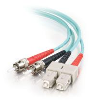
This USA made 0M3 Duplex Multimode Fiber Optic Cable is ideal for connecting 10GBase-SR, 10GBase-LRM, SFP+ and QSFP+ tranceivers for 10 gigabit network connections. This cable has a 0FNR-rated jacket allowing it to be used in a riser application. This cable also provides backward compatibility with existing 50/125 equipment and the performance headroom required to support LED and VCSEL laser light sources, and 10 gigabit ethernet applications.
