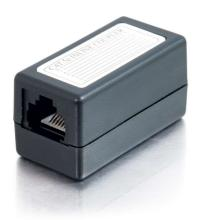
This coupler provides a female-to-female feed-through connection to extend the length of two Cat5E patch cables. Capable of handling LAN speeds up to 100 Mbps, this coupler meets TIA/EIA 568A specifications and is Power Sum Certified. Use for straight-through RJ45 Cat5E data applications.
