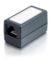
This coupler provides a female-to-female feed-through connection to extend the length of two Cat5E patch cables. Capable of handling LAN speeds up to 100 Mbps, this coupler meets TIA/EIA 568A specifications and is Power Sum Certified. Use for straight-through RJ45 Cat5E data applications.
