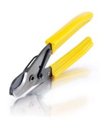
This tool cuts RG58 and RG6 coaxial round cable. Its curved cutting blades maintain cable geometry for a more precise cut. Cushioned grip handles provide comfort during multiple cuts while the locking latch keeps the tool closed in the pouch. Plus, steel-reinforced center conductors can be trimmed with the tool's bolt-cutting holes.
