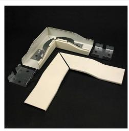
Wiremold 2400 series raceway is a single compartment raceway designed for communication or power applications and ideal for use in classrooms, offices, and hotel applications, or anywhere a small low profile raceway is needed. 90 degree flat corner elbow provides 2in cable bend radius for fiber optic and UTP/STP cable installations. Ideal for lay-in or pull-through installations. Couplings included.
