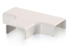
This tee is the ideal solution for making a right angle branches and connecting three pieces of raceway. The tee attaches to the end of three pieces of raceway and allows cabling to make a right angle turns. Available in standard colors which match the raceway, this tee features a smooth plastic finish, which is paintable with latex paint, and is designed to work with 2800 series raceway.
