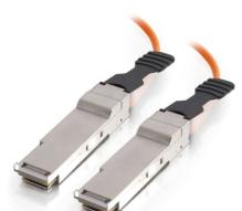
These cables are designed to support long length interconnects between active network equipment in data center and enterprise networking Infiniband applications. Our QSFP+ active optical cable assemblies are constructed using premium optical cable and feature active QSFP+ (SFF-8436) connectors with pull-tab ejectors for easy connection to equipment. These assemblies support up to 4x10G per lane for up to 40Gb, meeting or exceeding current standards specifications.
