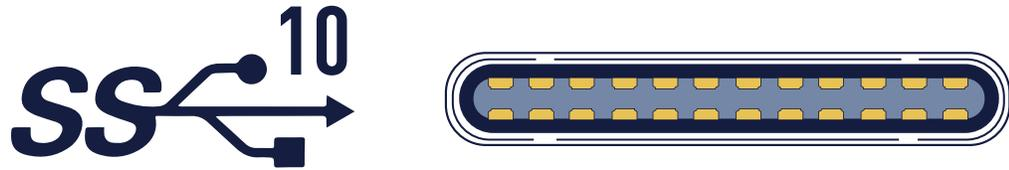
*Illus USB Type-C Superspeed + 10Gbit/s port tration of USB Type-C connector pin configuration*
