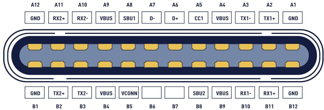
Illustration of USB Type-C connector pin configuration
