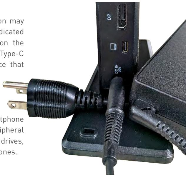
*Self Powered USB Type-C docking station showing proprietary power connection, USB Type-C monitor and DisplayPort ports.*
