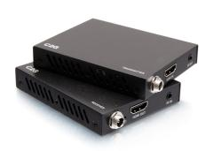
The HDMI over Cat Extender Box Transmitter to Box Receiver - 4K 60Hz allows a 4K HDMI source to be extended up to 131ft to a 4K display using a single Cat6/6a Ethernet cable. This is an ideal solution where HDMI video and audio in conference rooms. classrooms, lecture halls, and many other installation needs are far beyond the length limitations of standard HDMI cabling.
