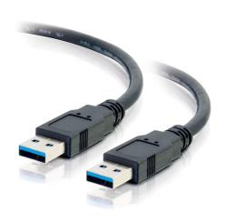
Just plug-and-play for hard drive enclosures, printers, modems, cameras, and other SuperSpeed USB peripherals. This cable provides a transfer rate of up to 5 Gbps when connected with a USB 3.0 compliant host and device. Foil and braid shielding reduces EMI/RFI interference and twisted pair construction helps reduce crosstalk thus ensuring SuperSpeed, error-free data transfer. Protective overmolded connector is color-coded blue to highlight USB 3.0 connectivity compatibility.
