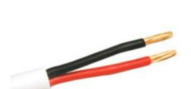
This is the right cable to install audio throughout your house. Made from 41 strands of 99.9% high-purity copper, this speaker wire is very flexible and less likely to kink during installation. CL2-rated for use inside walls, this wire features a flame-retardant white PVC jacket that helps to diminish the potential of fire spreading between floors.
