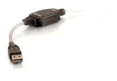
This USB active extension cable actively buffers the incoming and outgoing signals to ensure compliance with the USB 2.0 specification for electrical and timing minimums. Both low and high speed USB devices will function equally well with this USB active extension cable. This cable is ideal for electronic whiteboard applications when the distance is greater than 5 meters.
