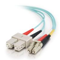
This OM3 Duplex Multimode Fiber Optic Cable is ideal for connecting 10GBase-SR, 10GBase-LRM, SFP+ and QSFP+ tranceivers for 10 gigabit network connections. This cable has a OFNP-rated jacket allowing it to be used in a plenum application. This cable also provides backward compatibility with existing 50/125 equipment and the performance headroom required to support LED and VCSEL laser light sources, and 10 gigabit ethernet applications.
