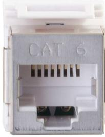
Designed for superior performance that meets or exceeds industry standard Category 6/Class E according to TIA/EIA 568B 2.1 and ISO/IEC 11801. This panel-type shielded RJ45 jack comes standard with 50 µinch gold plating on the jack contacts. The 2-piece shielded cover is designed for easy cable installation and protection from external radiated noise. Use for any unloaded keystone wall plate or patch panel.
