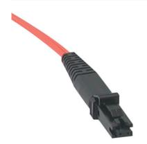
With MTRJ to ST termination, this high quality fiber optic patch cable is specifically designed for ethernet, multimedia, or communication applications. The MTRJ connector features an easy-to-use latch-type design similar to the RJ connector on a Cat5 patch cable, and is half the size of the SC connector. With its small footprint design, the MTRJ connector can increase the port density.
