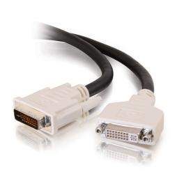
This precision-engineered cable is fully compliant with the DVI standard defined by DDWG (Digital Display Working Group). The DVI-I dual link configuration provides enough bandwidth for resolutions up to 2048 x 1536 pixels and allows high speed transmission up to 9.9 Gbps. Three analog 30 AWG coaxial lines enable high speed analog transmission.
