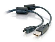
The Ultima USB cable optimizes style, quality, and value in a cable specially designed for high performance. USB devices with the mini-b port, and this cable will deliver high speed data transfer up to 480 Mbps. heavy duty 22 AWG power wires provide the proper current to your USB device. Dual foil and braid shielding reduces EMI/RFI interference while twisted pair construction helps reduce crosstalk thus ensuring high speed, error-free data transfer.
