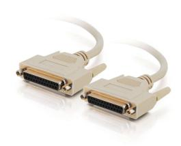
Place your serial printer or modem wherever you want with this economical DB25 extension. Or extend existing serial or parallel cables to connect through a switchbox or buffer or to connect to a modem. Remember that all 25 lines connect straight through pin-to-pin. Each cable is foil shielded for EMI/RFI protection, and is available fully molded with thumbscrew connectors for a fast, easy connection every time.
