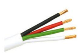
This is the right cable to install audio throughout your house. Made from 65 strands of 99.9% high-purity copper, this speaker wire is very flexible and less likely to kink during installation. CL2-rated for use inside walls, this wire features a flame-retardant white PVC jacket that helps to diminish the potential of fire spreading between floors.
