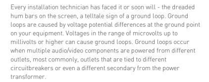
Ground loops manifest themselves in the form of hum bars called herringbone (diagonal lines on the screen) and AC beat (a wide, barely visible bar that rolls from the bottom to the top of the screen). Often you can hear the ground loop as the noise on the video encroaches on the audio signal.
