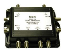
New generation DBS systems view and receive signals from satellites in multiple orbital locations to provide HDTV programming and local-to-local television programming. This multiswitch takes the signals from two dual LNBs and the signal from an off-air antenna or cable TV and distributes them to four satellite receivers. Satellite and off-air signals are separated at the DSS receiver using a diplexer. This multiswitch is weatherproof so you may mount it outdoors.
