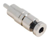
Quickly customize the length of your home theater or broadcast video cables with these connectors. Nickel-plated brass provides years of reliable service. These connectors are a breeze to install and more reliable than traditional hex crimp RCA connectors. Simply prepare 3- or 5-conductor miniature coax cable using the stripping tool (item #40998), insert the centerpin and compress it with the 3-in-1 compression tool (item #38011).
