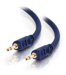
This cable is specifically designed to provide quality signal transfer for mono audio and data transfer applications. It features two 27 AWG oxygen-free copper conductors, a drain wire, an aluminum foil shield to prevent unwanted EMI/RFI interference, and fully molded, gold-plated connectors providing strain relief for a quality connection.
