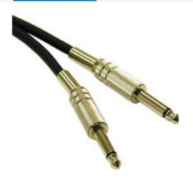
Use this 1/4in to 1/4in cable to connect unbalanced line outputs to unbalanced line inputs. This pro-audio cable is made from 22 AWG twisted pair audio cable under an aluminum foil shield and 60% copper braid for maximum shielding from noise. The highly flexible 7mm PVC jacket reduces the risk of the cable kinking and damaging the conductors.
