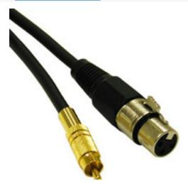
Use this XLR to RCA cable to connect balanced line outputs to unbalanced line inputs. This pro-audio cable is made from 22 AWG twisted pair audio cable under an aluminum foil shield and 60% copper braid for maximum shielding from noise. The highly flexible 7mm PVC jacket reduces the risk of the cable kinking and damaging the conductors.
