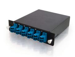
Small form factor: 1.125in x 5.125in x 4.5in. This breakout module provides the mechanical distribution of the 12-strand MTP/MPO connector. Housed in a rugged steel enclosure guaranteed for life, this durable module arrives fully loaded with the preterminated and tested MTP/MPO breakout harness. It is shipped with a test report that can assist in calculating the optical budget.
