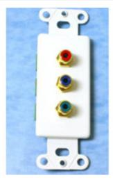
Add the finishing touch to your home theater installations. This insert is stamped from 20 gauge steel and painted to match your room decor. Use it in standard electrical boxes or mud rings, and with standard decorative wall plates for easy installation. With RCA jacks on the front and a screw-terminal block on the back, this insert is simple to install and use.
