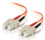
With SC to SC termination, this high quality fiber optic patch cable is specifically designed for fast ethernet, fiber channel, ATM and gigabit ethernet applications. The SC connector features a push-pull locking system. The LSZH jacket is composed from materials that lessen the smoke and halogen emissions when the cable is exposed to extreme temperatures.
