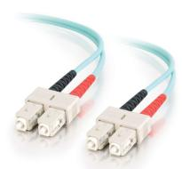
This OM3 Duplex Multimode Fiber Optic Cable is ideal for connecting 10GBase-SR, 10GBase-LRM, SFP+ and QSFP+ tranceivers for 10 gigabit network connections. This cable has a OFNP-rated jacket allowing it to be used in a plenum application. This cable also provides backward compatibility with existing 50/125 equipment and the performance headroom required to support LED and VCSEL laser light sources, and 10 gigabit ethernet applications.
