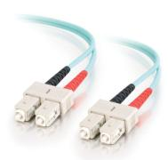
This OM3 Duplex Multimode Fiber Optic Cable is ideal for connecting 10GBase-SR, 10GBase-LRM, SFP+ and QSFP+ tranceivers for 10 gigabit network connections. This cable has a 0FNP-rated jacket allowing it to be used in a plenum application. This cable also provides backward compatibility with existing 50/125 equipment and the performance headroom required to support LED and VCSEL laser light sources, and 10 gigabit ethernet applications.
