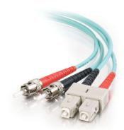
This OM3 Duplex Multimode Fiber Optic Cable is ideal for connecting 10GBase-SR, 10GBase-LRM, SFP+ and QSFP+ tranceivers for 10 gigabit network connections. This cable has a 0FNP-rated jacket allowing it to be used in a plenum application. This cable also provides backward compatibility with existing 50/125 equipment and the performance headroom required to support LED and VCSEL laser light sources, and 10 gigabit ethernet applications.
