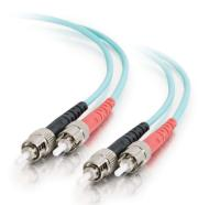
This OM3 Duplex Multimode Fiber Optic Cable is ideal for connecting 10GBase-SR, 10GBase-LRM, SFP+ and QSFP+ tranceivers for 10 gigabit network connections. This cable has a OFNP-rated jacket allowing it to be used in a plenum application. This cable also provides backward compatibility with existing 50/125 equipment and the performance headroom required to support LED and VCSEL laser light sources, and 10 gigabit ethernet applications.
