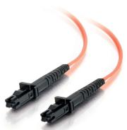
With MTRJ to MTRJ termination, this high quality fiber optic patch cable is specifically designed for ethernet, multimedia, or communication applications. The MTRJ connector features an easy-to-use latch-type design similar to the RJ connector on a Cat5 patch cable, and is half the size of the SC connector. With its small footprint design, the MTRJ connector can increase the port density.
