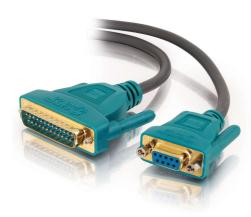
This Ultima cable optimizes style, quality, and value in a cable specially designed for high performance. 28 AWG conductors are insulated in polypropylene to minimize crosstalk, ensuring high speed, error-free transmission. An aluminum undermold shield assists in reducing interference to meet FCC requirements, while a 360° solder-to-connector shell and cable braid create an end-to-end shielding solution for a noise-free connection.
