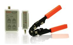
This kit includes an RJ45 crimper, and a UTP cable tester. The crimping tool cuts, strips and crimps RJ45 connectors onto unshielded twisted pair cable. The cable tester quickly identifies correct or incorrect wiring, reversed or open, for EIA/TIA-568A, EIS/TIA-568B, AT<(><<)>(><(>&<)>(<<<>>)>1 258, 10Base-T ethernet and token ring.
