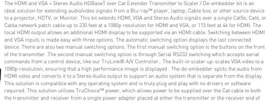
Note: Stranded Cat5e/6/6a patch cables may be used for HDMI extension applications up to 230ft. Shielded, solid conductor Cat6 or HDBaseT Certified Cat6a network cabling is recommended for applications where the category cable must be coiled, is run near other high-frequency signaling cables, or in high EMI/RFI environments. For best performance use a Cat6 Solid Shielded Patch Cable or anHDBaseT Certified Cat6a Patch Cable.
