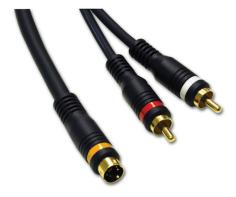
Carefully designed dual 75 Ohm precision video conductors ensure optimal video quality. Individually shielded Y (luminance) and C (chrominance) conductors are combined with an overall aluminum foil and OFC braid shield to protect against radio frequency interference (RFI) and electromagnetic interference (EMI). This cost-effective high-performance cable ensures maximum video quality when compared with s-video cables typically included with consumer electronics products.
