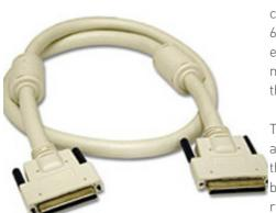
This Ultra2/Ultra3 LVD/SE external VHDCI (Very high density Cable Interconnect) cable features 28 AWG double-shielded twisted-pair cabling, ferrites and 0.8mm 68-pin molded connectors to reduce EMI/RFI interference. Designed to meet or exceed SCSI specifications, this cable is primarily used to connect advanced SCSI multiport applications to RAID controllers, and is built with the offset connector so that it may be used in stacking environments.
