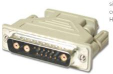
Updated version of item #28278, 13W3 Male to HD15 VGA Female Pinning Adapter. Has revised signals and a resistor and therefore is compatible with the newer Sun® systems. This adapter connects Sun workstations to monitors, and Sun workstations to the new Sun monitors that have an HD15 VGA connector. Do not use with SGIs. Functionally equivalent to Sun® #130-3034.
